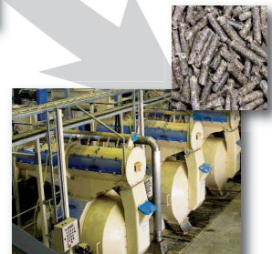
Pelleting machine: 12 t/h, 8 mm, low maintenance cost.
