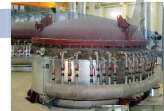
Juice purification with candle filters and press filters: improved sugar yield and sugar quality (partnership).
