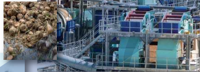
Washing plant with drum washers: high capacity, low maintenance, low water flows, high washing efficiency: final tare down to 0,2 % O.B.
