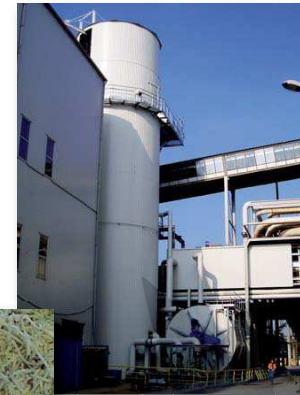
Tower Diffusers: high sugar extraction, low draft, minimal space.
